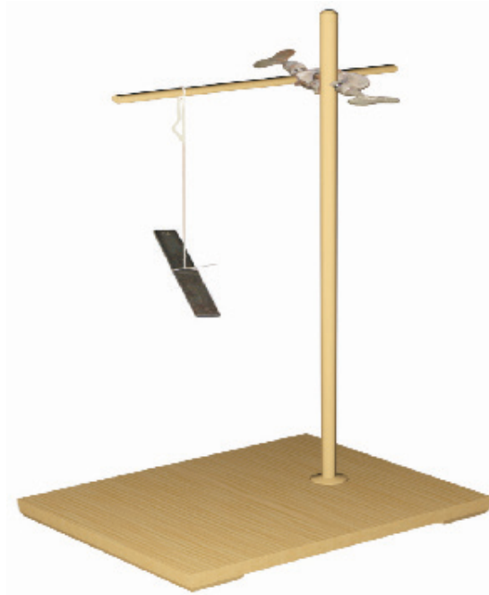
Fig 10.9 A freely suspended bar magnet always comes to rest in the same direction
